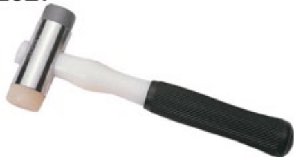
Soft faced hammer. The head is supplied complete with 38mm ø faces of soft plastic and nylon. The unbreakable nylon handle has a nonslip PVC grip. 72028: nylon face (spare part) 72029: soft plastic face (spare part)
