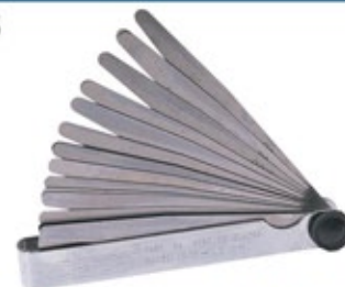
20 blade metric feeler gauge set. L=100mm. Sizes: 0,05 - 1,0mm.
