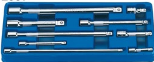
9 pc 1/4" 3/8" & 1/2" square drive wobble extension bar set. 1/4" square drive: 50, 100 and 250mm long 3/8" square drive: 45, 75, 150 and 230mm long 1/2" square drive: 125 and 250mm long
